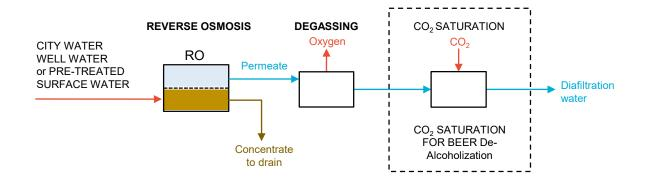
**Diafiltration** water should be **produced by RO. Degassing** is needed for extended shelf life of the final product. For most types of feed waters **Energy Saving membranes (ESPA) and CPA** are sufficient to provide high quality diafiltration water.
