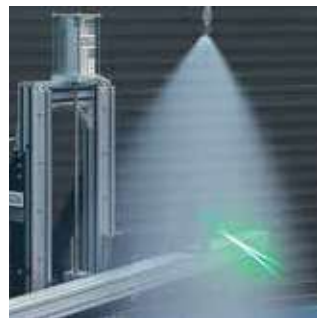
Figure 13: Droplet size measurement
