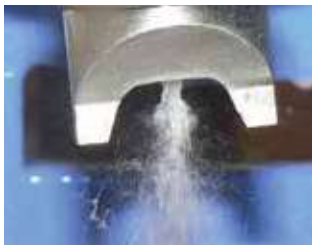
Figure 16: Atomization of gelatin with a Lechler ViscoMist twin-fluid nozzle
