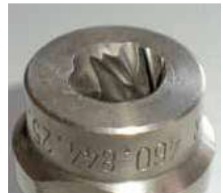
Figure 19: Wear of a full cone nozzle
