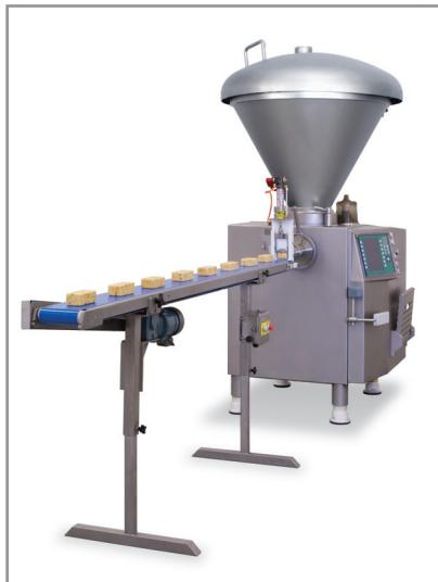
ment. The Vemag Cheese Block Former extrudes exact-weight cheese blocks with consistent dimensions. It is equipped with a cutoff device to control the length of the product and ensure clean, even edges. The extruder is designed for easy changeover from one shape to another. This innovative solution eliminates waste by repurposing cheese trim, ends, scraps and other pieces to produce cheese blocks. A common application for this system is the production of cheddar cheese blocks for retail.
