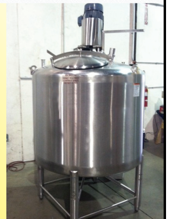
SST-104-01C: APV Model DTCB, 330 GALLON SINGLE SHELL HIGH SHEAR MIXING TANK. S/N-G6360, DOME TOP WITH MANWAY, CONE BOTTOM, 3HP HIGH SHEAR MIXER WITH SQUIRREL CAGE STYLE AGITATOR, 2.5" TRI CLAMP OUTLET.
