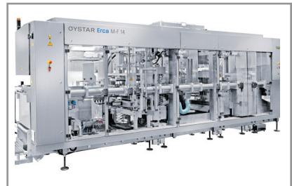
transports preformed containers up to 140mm in height and up to 2,500 grams in volume at speeds up to 57,600 units/hr. The system is lubrication-free, making it ideal for use in hygienic conditions including the production of dairy products.
