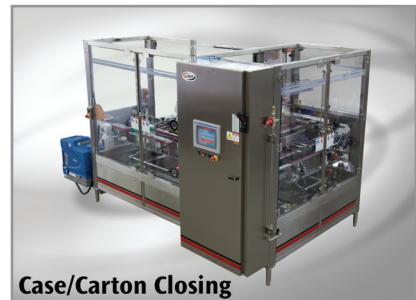
and makes precise adjustments to ensure square folding at speeds of up to 150 cartons per minute. No other carton closer in the world has this capability.
