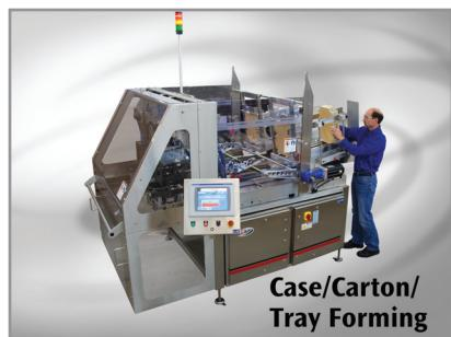
Delkor's best-selling Trayfecta® Former offers maximum flexibility for forming cases, cartons and trays using corrugated materials, paperboard or microflute. Tool-less changeovers between all these formats can be made in a matter of min-
