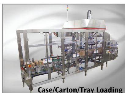
Delkor's loaders offer great flexibility to suit any product size and shape requirement with speeds of up to 700 containers/minute. The loaders are equipped to monitor product and case defects and discharge these defects from the machine without stopping production. The highly regarded Spot-Pak® loading system, which utilizes flat pads and shrink wrapping, is noted both for high productivity and its sustainability benefits. Delkor also offers case/carton loaders with integrated closers.
