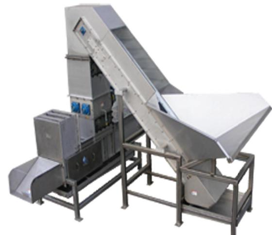
Designed specifically for removing liquids from aluminum cans, plastic bottles or other liquid containers
