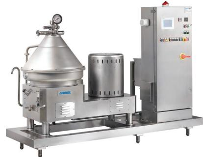
The **ANDRITZ** high speed clarifiers and separators are designed for liquid-based applications. In the Dairy Industry High centrifugal force and large surface area (disc stack) allow for the separation of liquids from liquids with removal of solids at the same time. Both clarifier (liquid-solid separation) and separator (liquid-liquid-solid separation) are offered for a wide range of capacities and processes.
