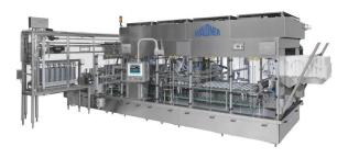
DOSOMAT MicroBio-Clean machines with cup/lid sterilization technologies for fresh and cultured dairy products are complete wash-down, CIP rated IP-65, USA dairy environment construction.
