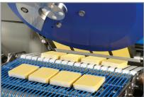
assist the production of perfect slices and consistent portions, while reducing product waste to near zero. Processors can simultaneously slice two four-inch logs at blade speeds up to 400-RPM. Touch-screen controls adjust slicing parameters and speed product changeovers. Interleave in stacks or shingles at up to 400 slices per minute.
