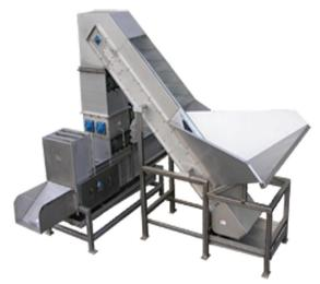
Designed specifically for removing liquids from aluminum cans, plastic bottles or other liquid containers
